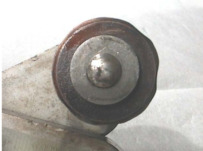
Original plain roller contact on scissor arm showing signs of uneven wear. The solution to this problem is to upgrade to ratchet rollers.
